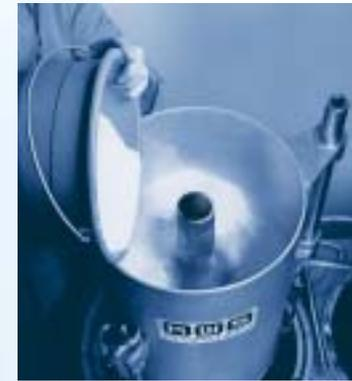
The variable speed mixer guarantees that the correct rotational speed for the specific investment process can be selected at all times.
