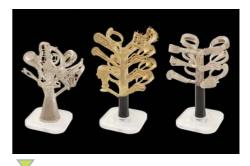
Direct casting using DigitalWax resins
